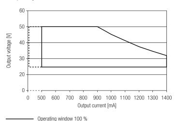
Make sure that the LED Driver is operated within the given window under all operating conditions, also in dimming operation. Otherwise certain limitations may occur. This is due to the nature of amplitude modulation dimming. The stated minimum output voltage shall not be undercut as this may cause the device to shut-down. In this respect, special attention needs to be paid to DC operation.
