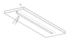
The width applicable to F22: 22~25mm The thickness of ceiling: 5~50mm
