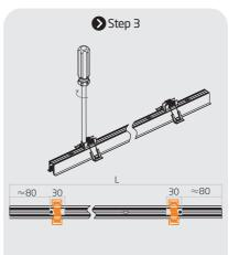
Unfold the spring a little and slide to groove of mounting profile.
