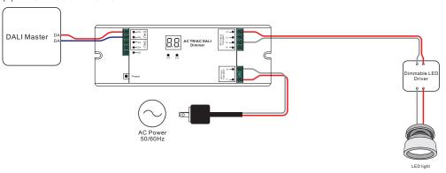
This phase dimmer adopts trailing edge dimming (reverse phase control), please make sure the connected loads support reverse phase control. Please refer to the user manual of the load or consult the supplier of the load.
