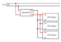
The diagram above is an example of the connection and may be different from the actual layout. Wires between the power supply, controller and LED modules should be as short as possible. Connecting more than one controller to the same power supply is not recommended. It may cause interference, visible on LED light sources. Controllers adapted to such work are available on special request.
