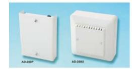
There are two versions of microphone: AD-260P and AD-260U. **AD-260P** has a sheet metal enclosure for surface mounting. **AD-260U** has a plastic enclosure for surface mounting or recessed mounting. It fits standard electrical housings.
