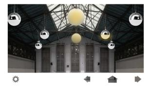
Custom1: Image of a room, the luminaries in the image can be turned on and off, by touching the luminary on the display. The display shows the current status of the lamp.
