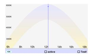
The DALI Display allows room-lighting based on the average daylight-curve using DALI DT8 luminaries (mode Tc). Depending on the current time the light changes to a warmer/cooler colour temperature.
