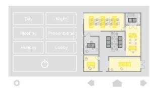
Custom2: Room-overview of an office, several scenes can be retrieved. In the room-plan the current light situation is displayed. The lighting of a room can be adjusted by pressing the room, or a scene-button.
