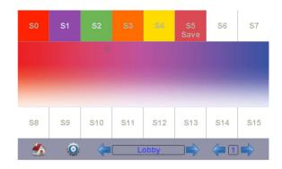
The DALI Display supports DALI DT8 RGB luminaries. The device allows to set RGB-values for scenes. During the colour selection the current settings are simulated by the active light-group, the settings can be saved afterwards. Using these scenes different colour-settings can be realized.
