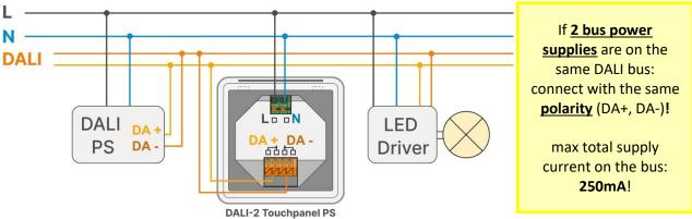
Figure 4 installation example DALI-2 Touchpanel PS with an additional DALI PS on the DALI bus
