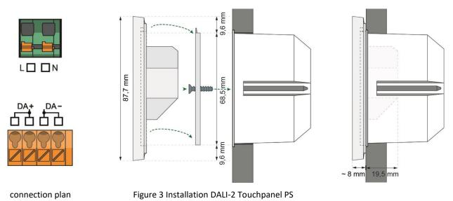
DALI-2 Touchpanel PS Touchpanel -> mounting plate -> flush-mounted box
