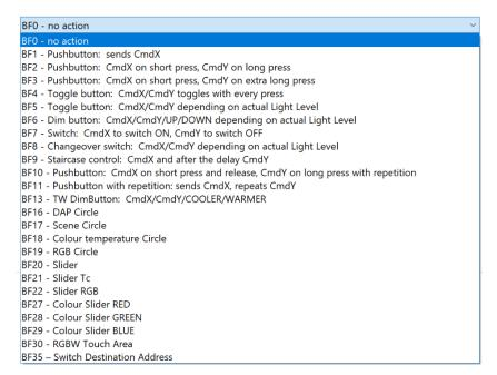
Figure 11 DALI-2 Touchpanel button functions
