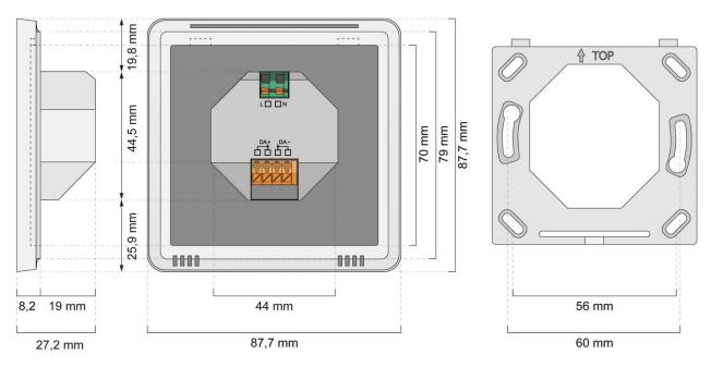
dimensions DALI-2 Touchpanel PS - Version with integrated DALI bus power supply
