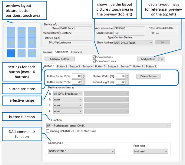
Figure 8 Application: Application Controller
