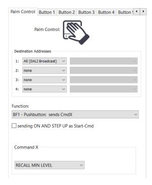
Palm control allows fast light control by placing the entire hand on the DALI-2 Touchpanel. Following buttons functions are available for palm control.
