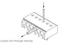
Loosen wire through twisting and pulling or using a Ø 1mm release tool
