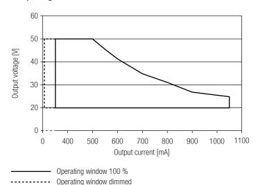
Make sure that the LED Driver is operated within the given window under all operating conditions, also in dimming operation. Otherwise certain limitations may occur. This is due to the nature of amplitude modulation dimming. The stated minimum output voltage shall not be undercut as this may cause the device to shut-down. In this respect, special attention needs to be paid to DC operation.
