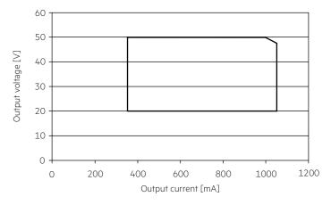
Make sure that the LED Driver is operated within the given window under all operating conditions. Coming below the specified minimum output voltage of the LED Driver may cause the device to shut-down.
