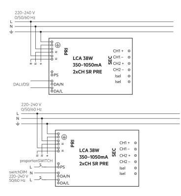
Device with loop through wiring function.
