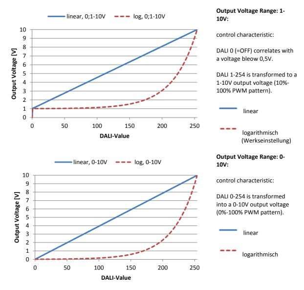
Note: the voltage values given in the control characteristics are valid only in the case that 10VDC are applied to the output
