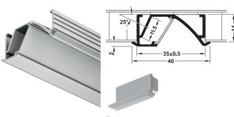
For panel thickness from 16 mm and > Area of application: above > Installation: For recess mounting
