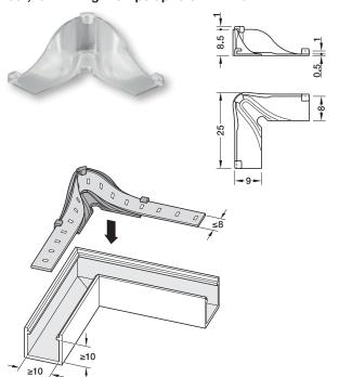
Bending instead of cutting allows creation of 90° illuminated frames without loss of light in the corners
