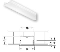
A = min. depth 10 mm for invisible LED points, with LED strip lights from 120 LEDs/m
