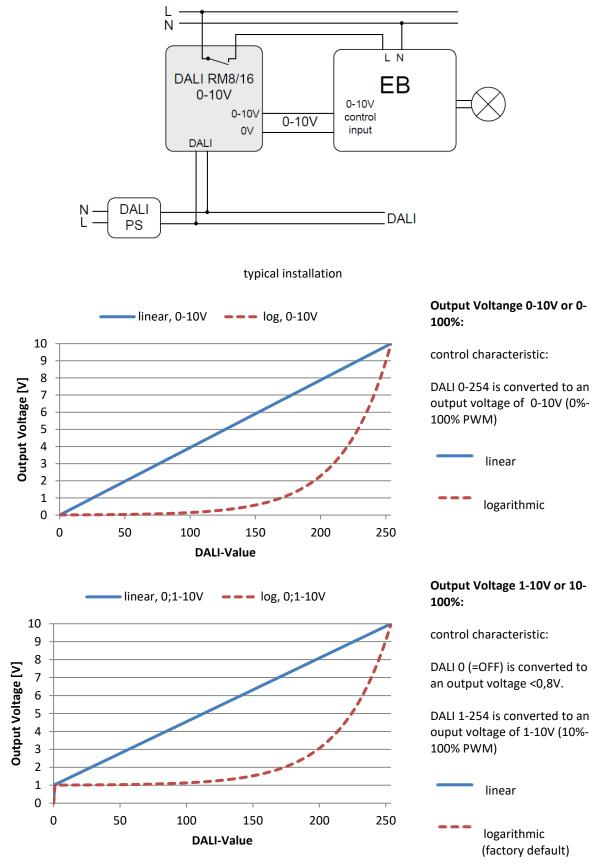
**Hint**: the voltage values in the characteristics are only valid if the device is supplied with 10V at the 0-10V output.
