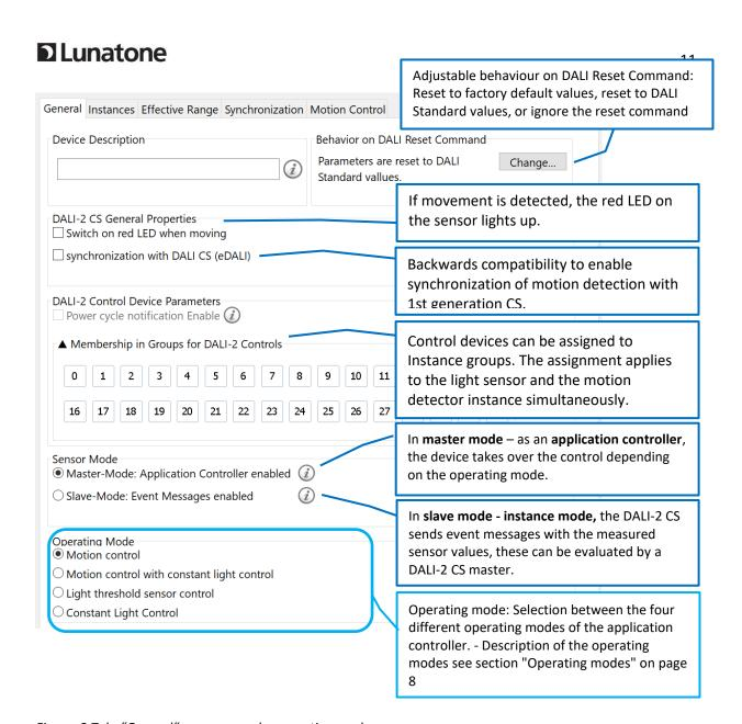
Figure. 2 Tab: "General" – sensor mode, operating mode
