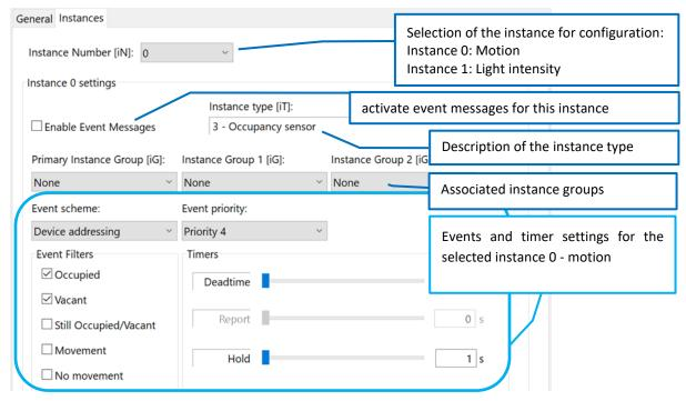
Figure. 8 tab: "Instances" – motion detector instance
