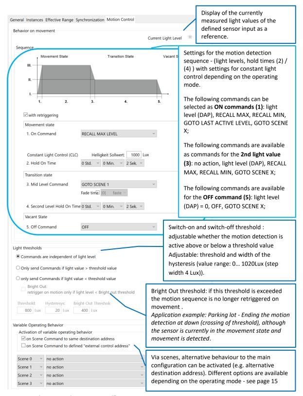
Figure. 5 Tab: "motion detection control"
