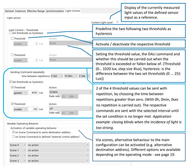
Figure. 6 Tab: "Light Control" -Operating Mode: without constant light control
