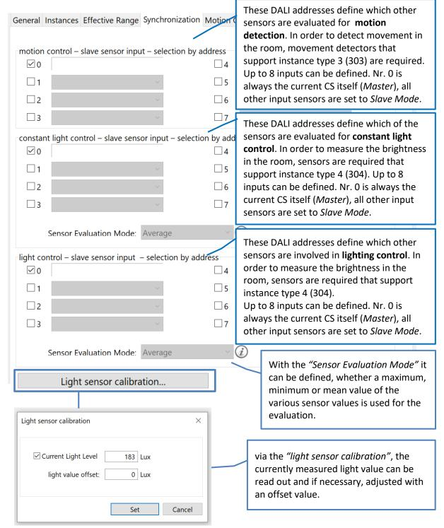
Figure. 4 Tab: "Synchronisation" - sensor inputs for measurement evaluation
