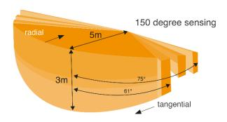
Figure 1 Detection area: X-Y cross section at 1m
