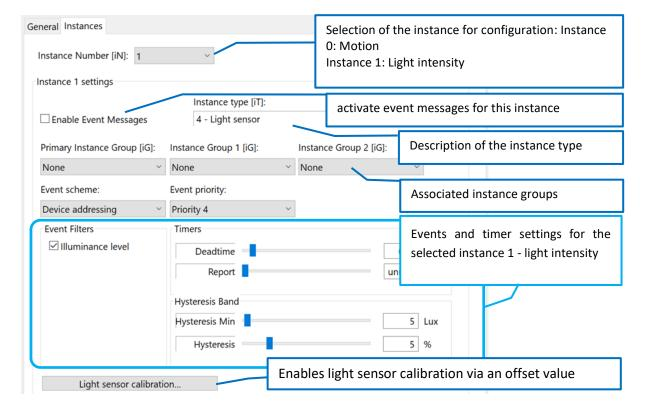
Figure. 9 tab: "instances" - light sensor instance
