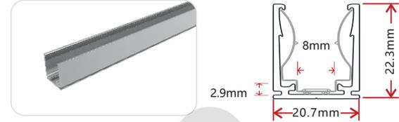
Note: Unless otherwise stated, the tolerance of the profile is ±0.5mm.
