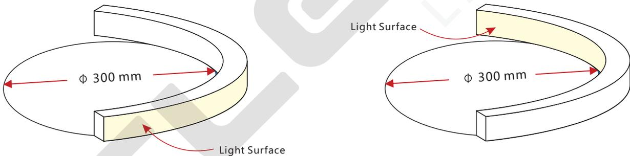
The light can only be bent along the light surface. Do not bend smaller than allowed minimum bend diameter.
