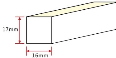
Note: Unless otherwise stated, the tolerance of the light is  $\pm 0.3\text{mm}$ .
