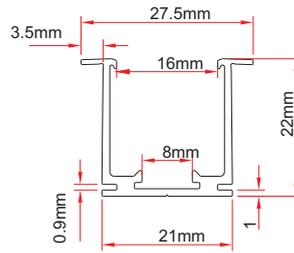
Note: Unless otherwise stated, the tolerance of the profile is  $\pm 0.5\text{mm}$ .
