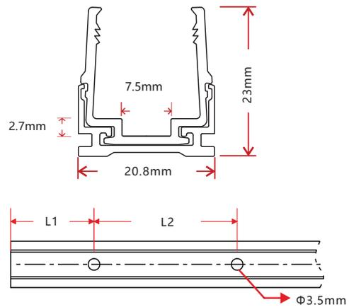
Note: Unless otherwise stated, the tolerance of the profile is ±0.5mm.
