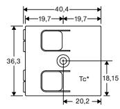
Mounting hole diameter: 3,5 mm
