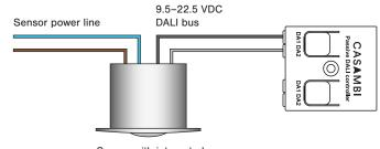
Sensor with integrated DALI power supply
