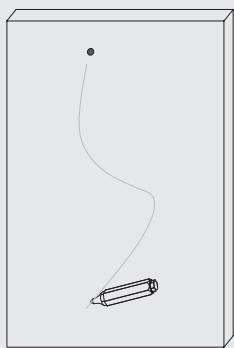
Mark the required shape on the mounting surface or print the sketch in the scale of 1:1 if complicated.
