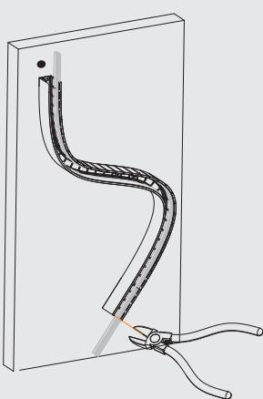
Adjust the serrate silicone tape and remove the redundant lengths at both ends.
