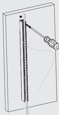
Get the front connector outside of profile and keep at least 10mm more apart. Fix the screw starting from the power input end.
