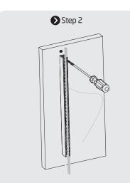
Get the front connector outside of profilel and keep at least 10mm more apart. Fix the screw starting from the power input end.
