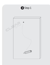
Mark the required shape on the mounting surface or print the sketch in the scale of 1:1 if complicated.
