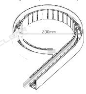
Min. Bending Diameter (Toothed Side outwards)
