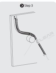
Use cylinder or disc-like object you have to assist with shaping.
