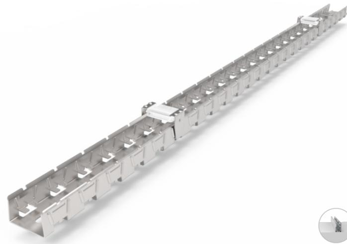
It's engineered for the safe and quick installation of F2010 Explosion Proof LED Strip. The design is smart enough to fix LED strip tightly, preventing it from falling off the mounting profile when vibration occurs. Accessories are available on demand for either screw mounting or strap mounting based on the site condition. The main structure, made of 316L stainless steel, makes it resistant to corrosion, suitable for environments where hazardous gas or dust exists and industrial workplaces.
