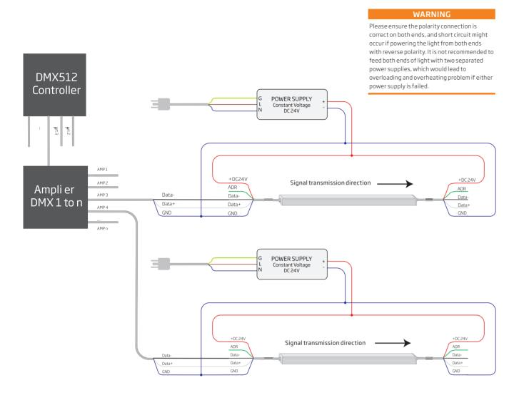
Please refer to the following wiring diagram with double-end feed to run length that is longer than max. running length for single-end feed but less than twice the value.
