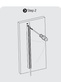
Get the front connector outside of profilel and keep at least 10mm more apart. Fix the screw starting from the power input end.
