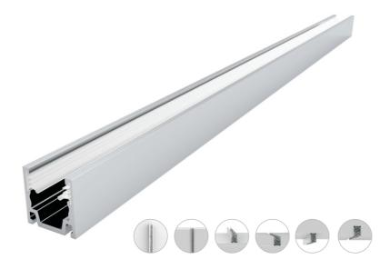
Specialized for the LED Flex Linear light, it was developed by combining the advantages of 6063 aluminum and elastic serrated tape. The inside elastic serrated tape as the grabbing force to keep continuous strong clamping force on the light body and protect the light from the damage caused by the large friction in the process of installation and dismantlement. It can stand max. 50 times of the light weight under -20~70°C and is easy to install and dismantle.
