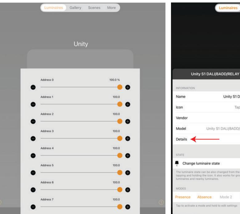
Hold your finger over the D1 icon to bring up dimming options. In this profile upto 8 DALI addresses are individually controllable. Addresses are listed from Address 0 (A0) to Address 7 (A7). The dimmers listed directly control the DALI devices based on what DALI address they have. In this way you can individually control upto 8 DALI addresses from D1. See next details for how to see what DALI devices have which address and how to change thier Address.
