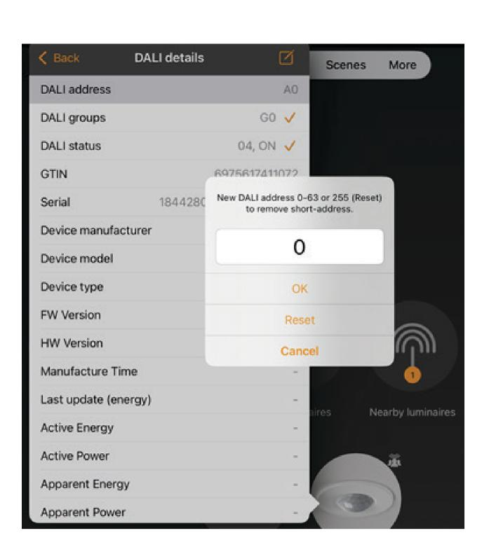
Select the Address you want to change the device too. A maximum of 8 Addresses (A0-A7) are useable in this profile. If you select an address that is already taken the system will assign the device with the current address to another address automatically. Return to the Details tab to see Address assignment.
