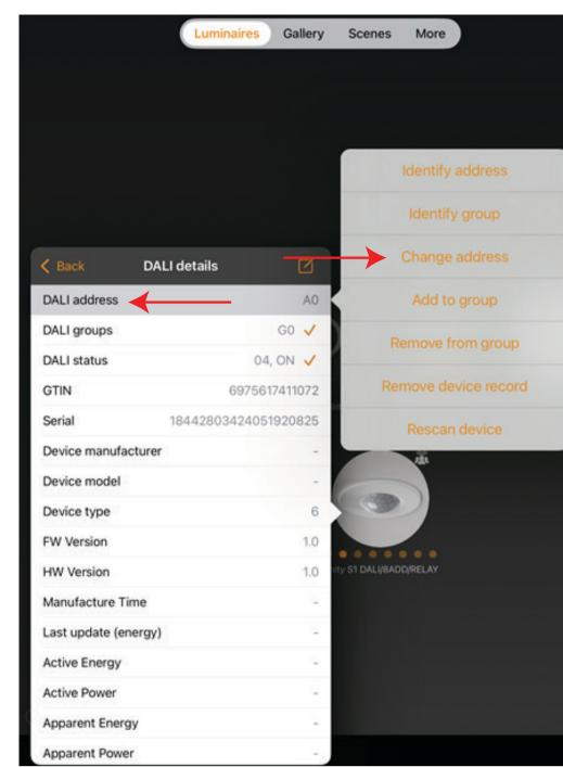
Tap on DALI Address. A box pops up showing available options. The most useful options are Identify the DALI devices Address, Identify Group, Change Address and Add or Remove from Group. Tap Change Address.
