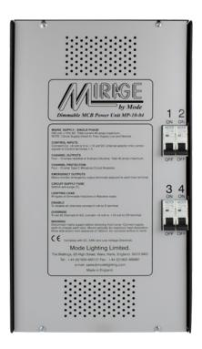
The Mirage MP-10-04 is a wall mounting, four channel, Dimmable Power Unit designed for the reliable, leading edge, mains dimming of tungsten resistive and LV inductive lighting loads. Each of the four circuits is rated at 10 amps resistive or 9 amps inductive load and is protected by a Type C Miniature Circuit Breaker (MCB).
