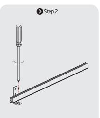
Fix side mounting bracket and mounting profile tightly by the screw.
