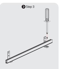
Repeat step 1 & step 2 for the remaining brackets and secure at least 2 locking points for each mounting profile, and the equal interval is more recommended.
