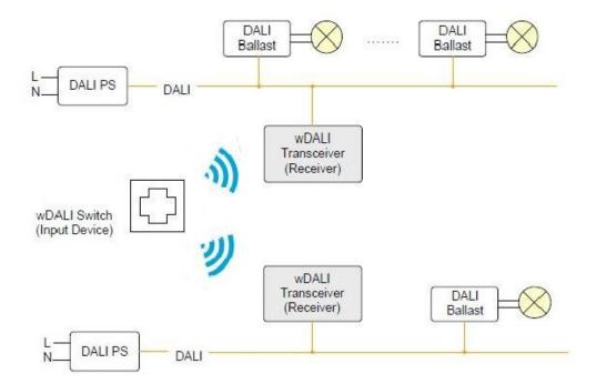
typical installaiton (one input device, simultanous conrol of multiple DALI-lines)
