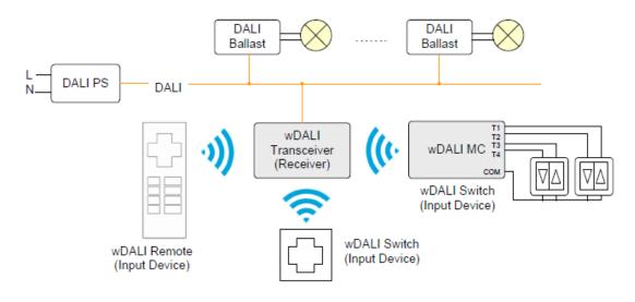
typical installation (several input devices, one transceiver)
