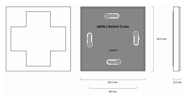
geometry wDALI Switch Cross (input device)
