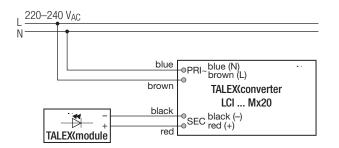
Secondary switching of LEDs is not allowed and may cause damage to the LEDs. The hot plug-in of LEDs during normal operation may result in current peaks of up to 50% above the typical output current.
