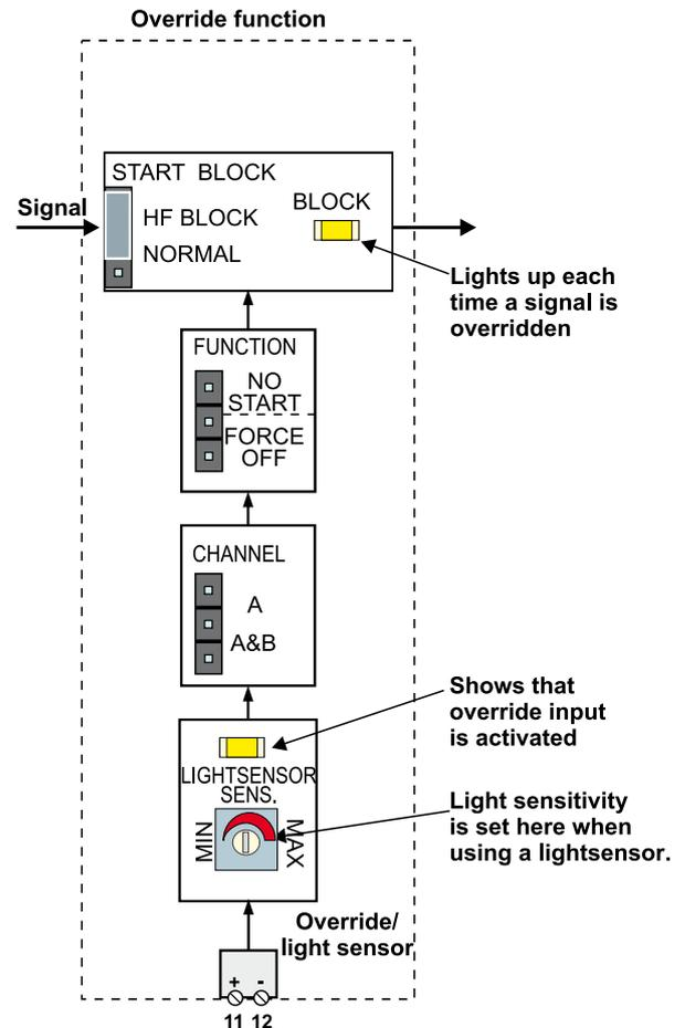
The **CHANNEL** jumper can be used to select whether you want just one channel (A) or both channels (A & B) to be activated by the blocking input. If the **TOGGLE function** mode is used it blocks channel A or channel B whenever the jumper is in position "A".
