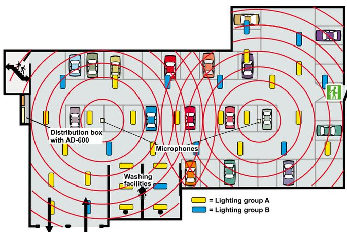
The old light fittings mean that the fluorescent tubes suffer from rapid wear if they are switched on and off without being allowed to cool down after switching off. Switching on fluorescent tubes when they are hot should therefore be avoided.
