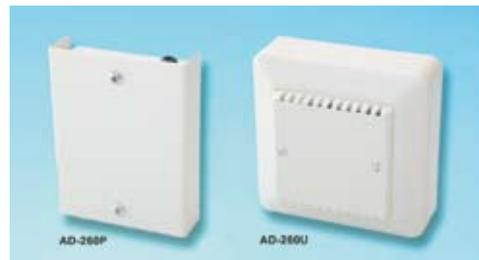
There are two versions of microphone: AD-260P and AD-260U. **AD-260P** has a sheet metal enclosure for surface mounting. **AD-260U** has a plastic enclosure for surface mounting or recessed mounting. It fits standard electrical housings. The sensitivity of the microphones to HF and LF ranges can be adjusted independently.
