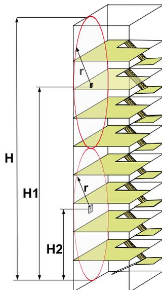
Example: AD-500 and single AD-260 microphone installed in a stairway.
