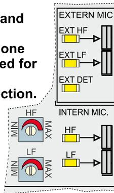
**Only external microphone connected for LF and HF detection.**
